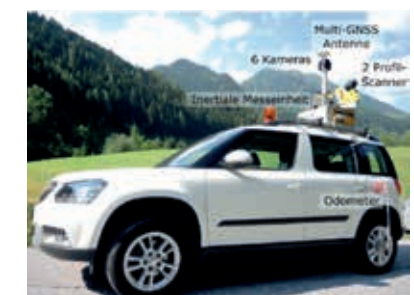
Abb. 2: Links: Komponenten eines Mobile Mapping Systems
